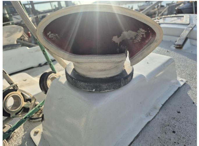
Damaged vent head
