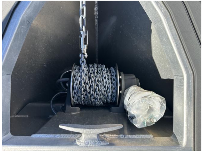
Drum anchor winch
