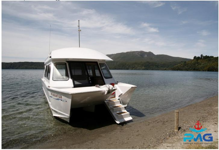
**Features include** Stable 3.6m beam: 3 x 20ltr tote tanks/motor: Boarding doors both sides: Bow steps pneumatically operated: Toilet cubicle with removable cassette toilet: 2 burner gas elements: Gas Califont for hot water: Sink: Wash down hoses bow and stern: Chain/rope anchor pack Anchor Capstan operated from Helm:
