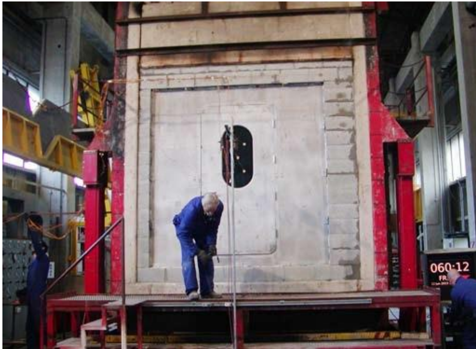
Exterior door immediately after 60 minute test up to 925 degrees Celsius
